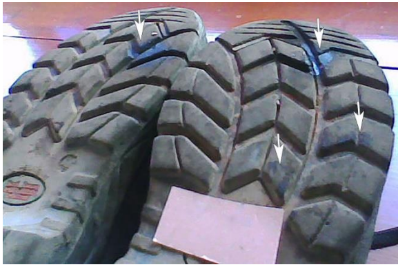
Fig. 4: Damage on shoes (indicated with arrows)
